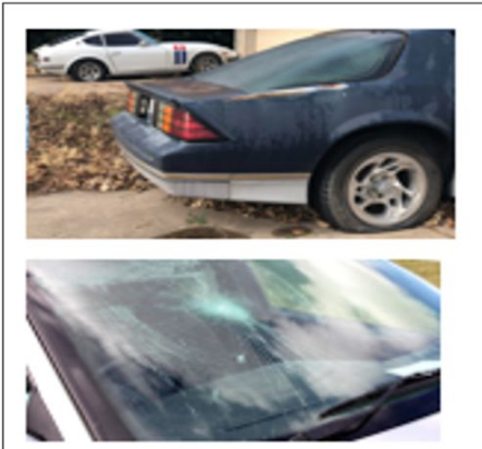
Inoperable isn't limited to the motor. Above are some examples; flat tire & broken windshield
